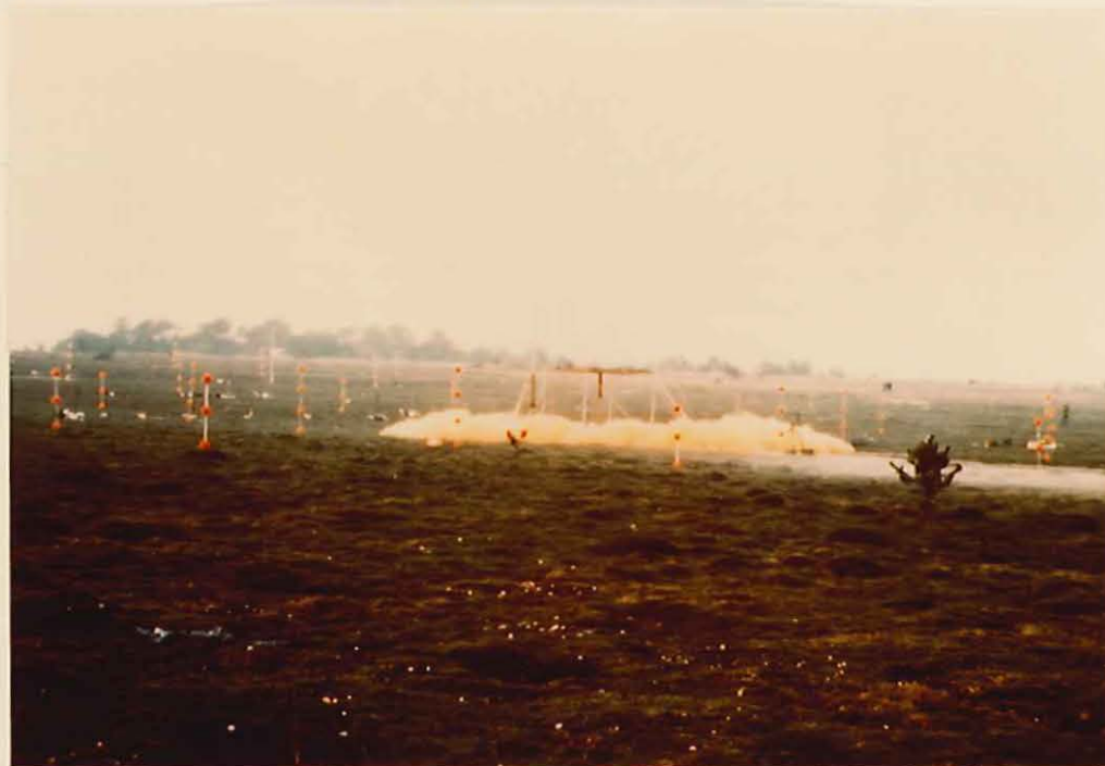
FIGURE 3(a) Collapse of Freon - 12 'puff' when there is little wind.
