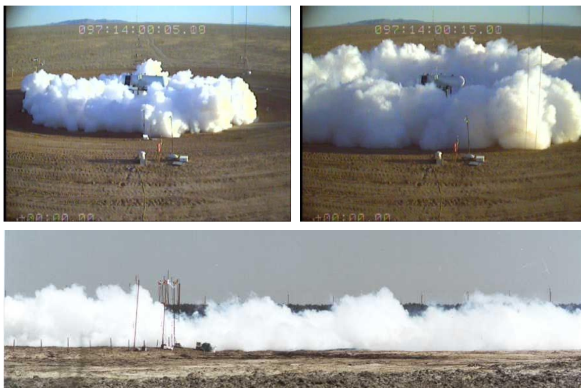
Figure 5 Top: Ammonia cloud dispersing 5 s (left) and 15 s (right) after release at Dugway Proving Ground during Jack Rabbit trials (Storwald et al., 2011, © UVU copyright 2011). Bottom: Ammonia released during large scale field trials undertaken by INERIS (Bouet, 1999, © INERIS copyright)
