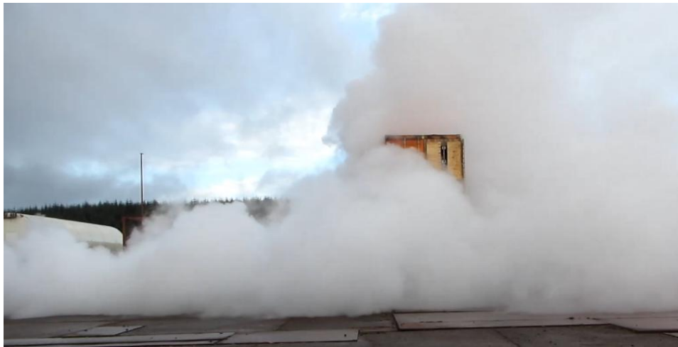
Figure 17 Carbon dioxide cloud dispersion around containers (Cleaver et al., 2016). Cloud motion is from left to right. Cloud builds up in front of the obstruction then travels round it and mixes in the lee downwind significantly increasing the depth of the cloud (© IChemE copyright 2016)
