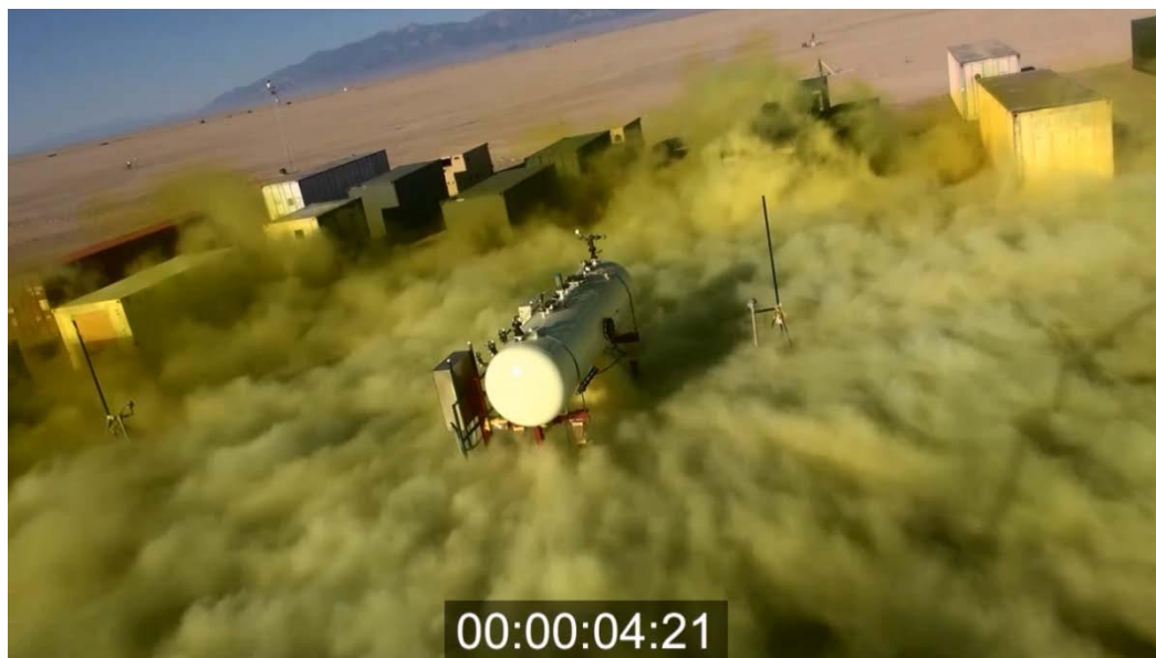
Figure 18 Image of a pressure-liquefied chlorine release from a rail car from Jack Rabbit II experimental Trial 4 (Byrnes et al., 2017, © UVU copyright)
