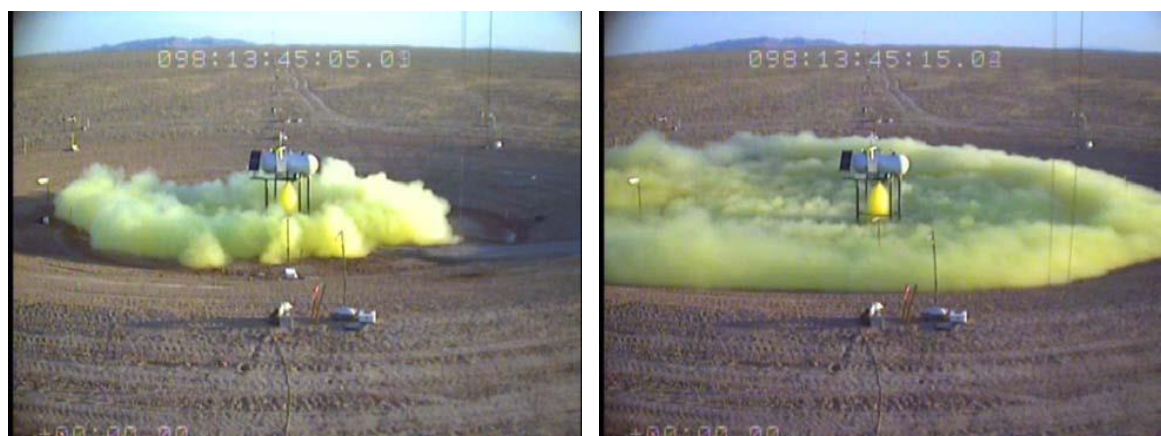
Figure 4 Chlorine cloud dispersing 5 s (left) and 15 s (right) after release at Dugway Proving Ground during Jack Rabbit trials (Storwald et al., 2011, © UVU copyright)
