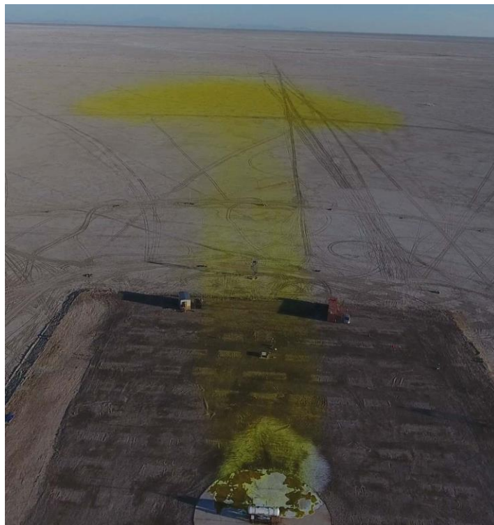
Figure 14 Mushroom-shaped cloud resulting from release of pressure-liquefied chlorine in the Jack Rabbit II Trial 7 (Byrnes et al., 2017, © UVU copyright)
