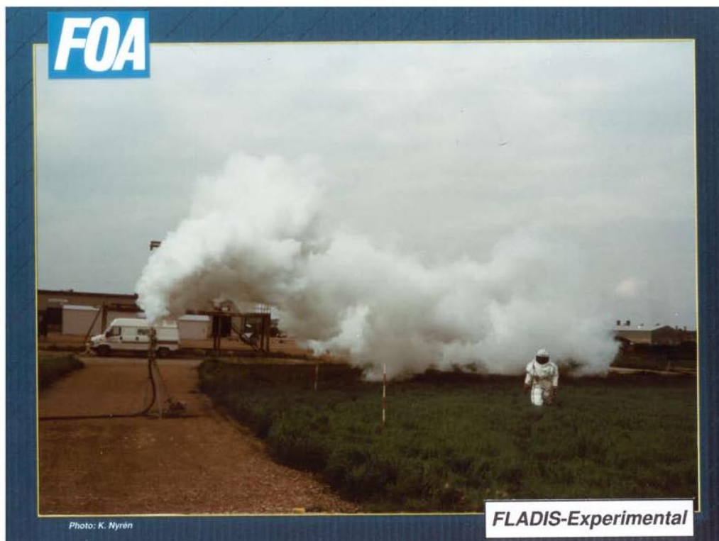
Figure 44 Example of a flashing release of ammonia from the FLADIS programme. Discharge rate is approximately 0.25 kg/s. Image from Nielsen et al. (1994, © K. Nyren copyright, FOI).
