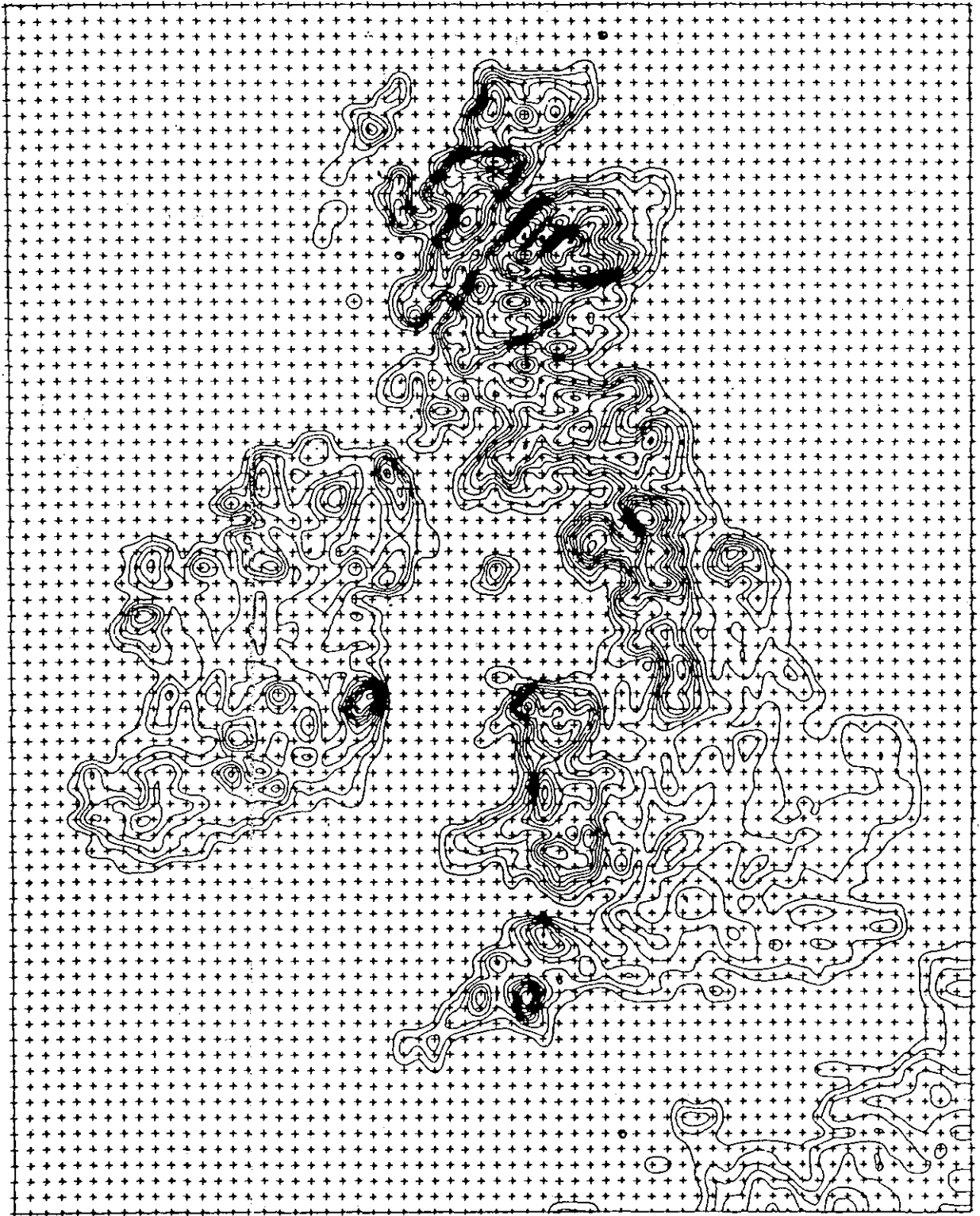
Fig.2.27 Model domain and orography for the Meteorological Office mesoscale model (from Golding 1987). Grid point spacing is 15km. Contours represent 50m steps.
