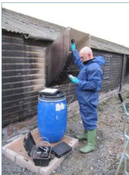
Figure 11 Upward pointing cowl at Glendevon Farm; figure taken from Hill et al. (2014), reproduced here with permission from Sniffer (private communication, 05/08/15).
