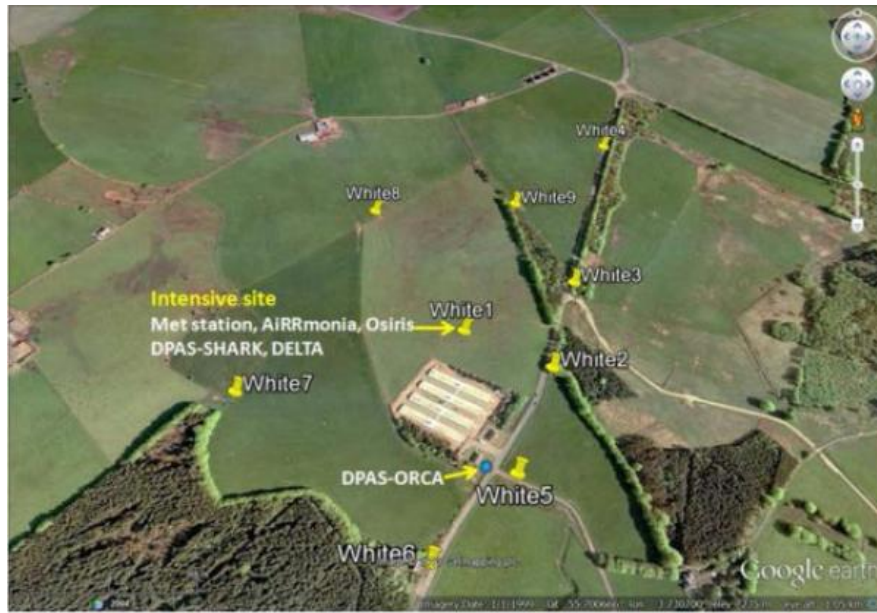
Figure 12 Whitelees Farm study area showing location of the onsite meteorological station (White 1) which is co-located with the continuous ammonia monitoring equipment; White 2 to White 9 indicate the locations of additional ammonia measurements; figure taken from Hill et al. (2014), reproduced here with permission from Sniffer (private communication, 05/08/15).
