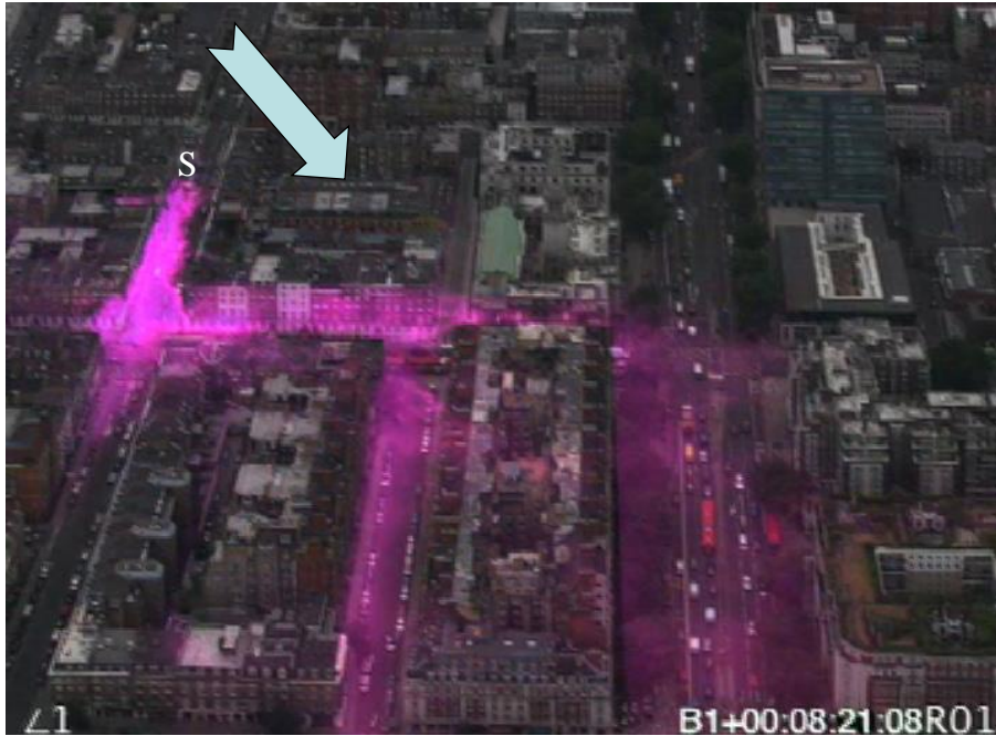
Figure 3.6. Smoke visualisation of pollutant exchanges at intersection in the DAPPLE field site in central London. False coloured image derived from wind tunnel flow visualisation study. The illumination is concentrated on the street canyons and pollutant that has been transferred to the external flow is not visible in this image. The source is at the point S and the wind at incidence to the street network. (DAPPLE, 2011)
