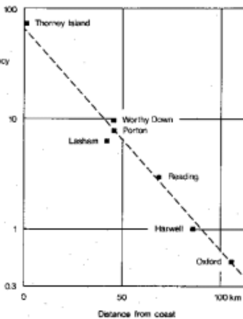
FIGURE A3.10 Progress inland of the sea-breeze fronts on the south coast of England (reproduced with permission from Simpson et al 1977). The diagram on the left shows the average progress; the graph on the right the progress for one particular breeze
