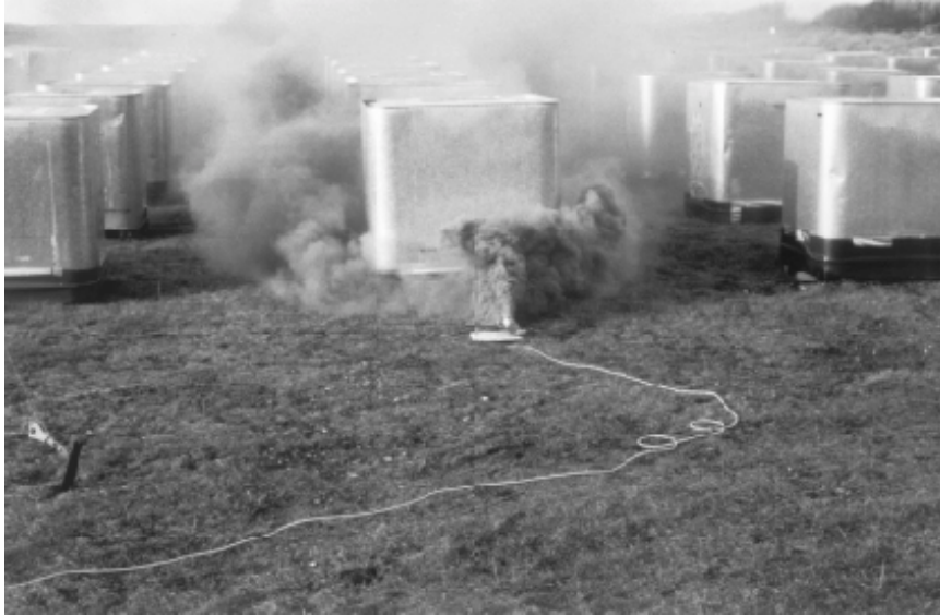
FIGURE 5.17 Entrainment of a ground-level plume into the horseshoe vortex system around the base of a cube in the front row of an array of 16% plan area density (Macdonald et al , 1998b, courtesy of Atmospheric Environment )
