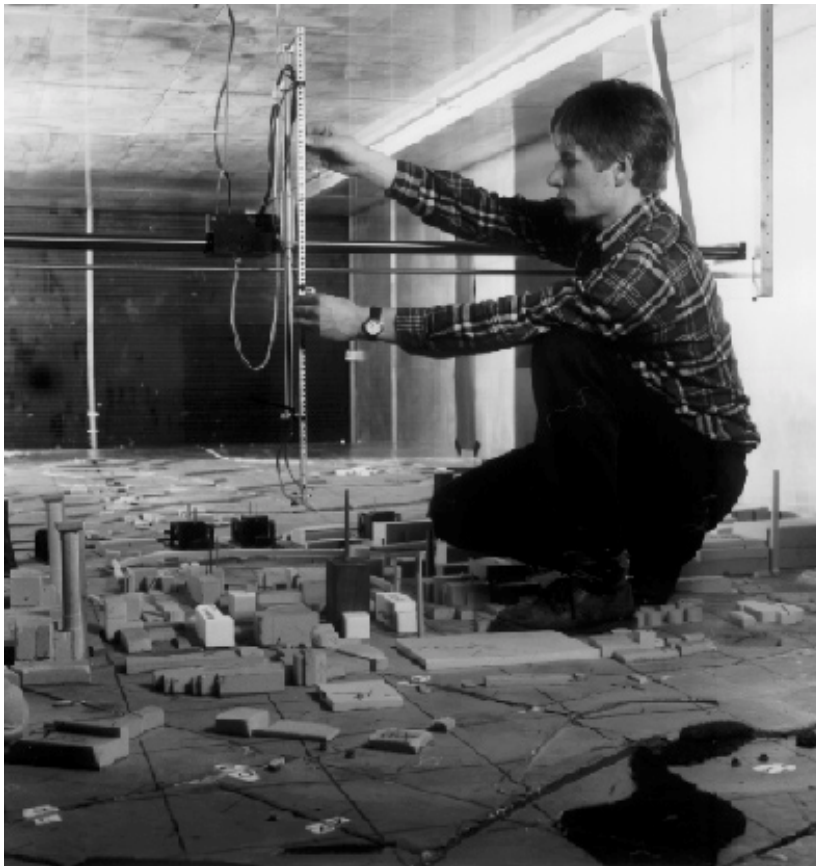
FIGURE 4.1 A detailed site model installed in an environmental wind tunnel
