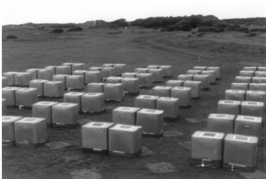
(b) Eight-row array of obstacles with width to height ratio W/H = 2 in the field; row spacing S/H = 2
