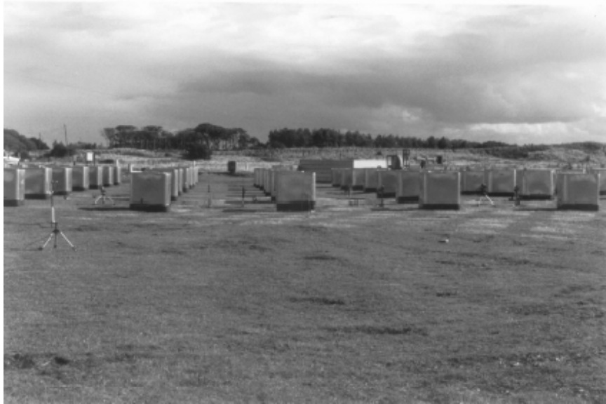
(a) Low-density array of obstacles ( \lambda_p = 6.25\% ) with wide obstacle spacing S/H = 3
