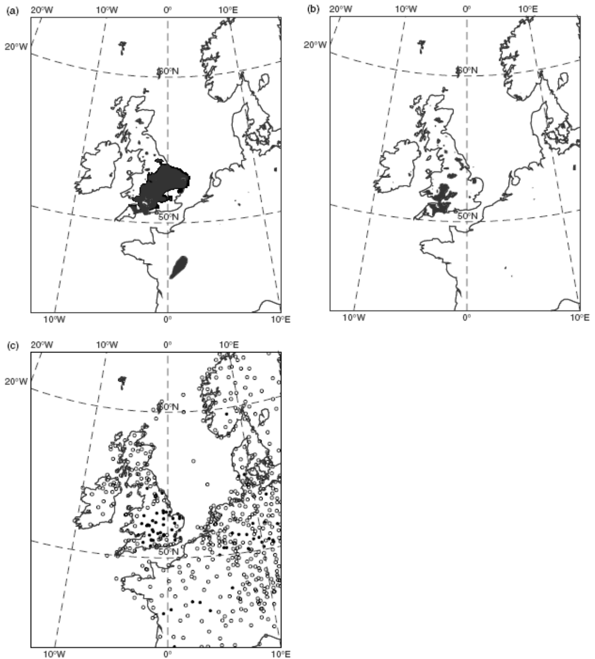
Figure 25. Forecasts of fog probability at 12:00 on the 22 nd of December 1998 from Clark et al. (2008). The shaded regions of images (a) and (b) indicate a probability greater than 0.4. Image (a) includes the assimilation of visibility observations into the model, whereas they were excluded from the trial in image (b). Image (c) shows where observations of visibility at 12:00 were made: shaded / open circles show visibility reports of less than / greater than 1 km respectively.
